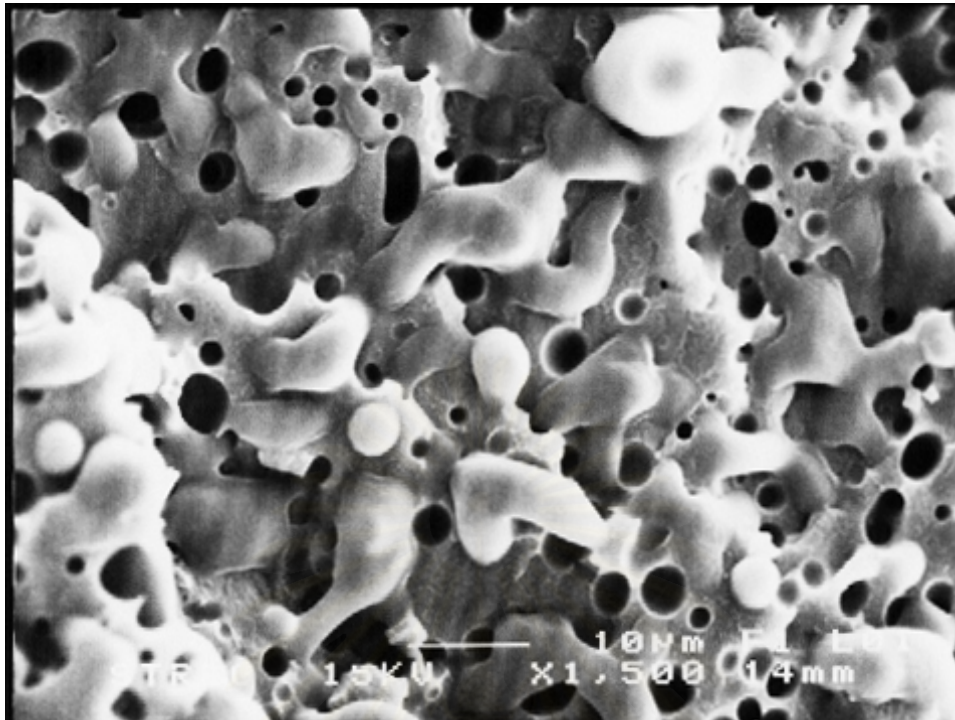
Figure 4.20 Scanning electron micrograph of PET/Buna3950 blend at 70/30.
