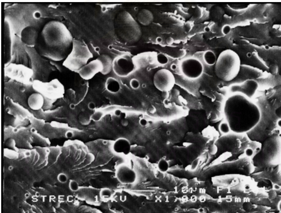
Figure 4.11 Scanning electron micrograph of PET/Buna3950 blend at 80/20, using 1 phr MAH grafted onto EPDM.
