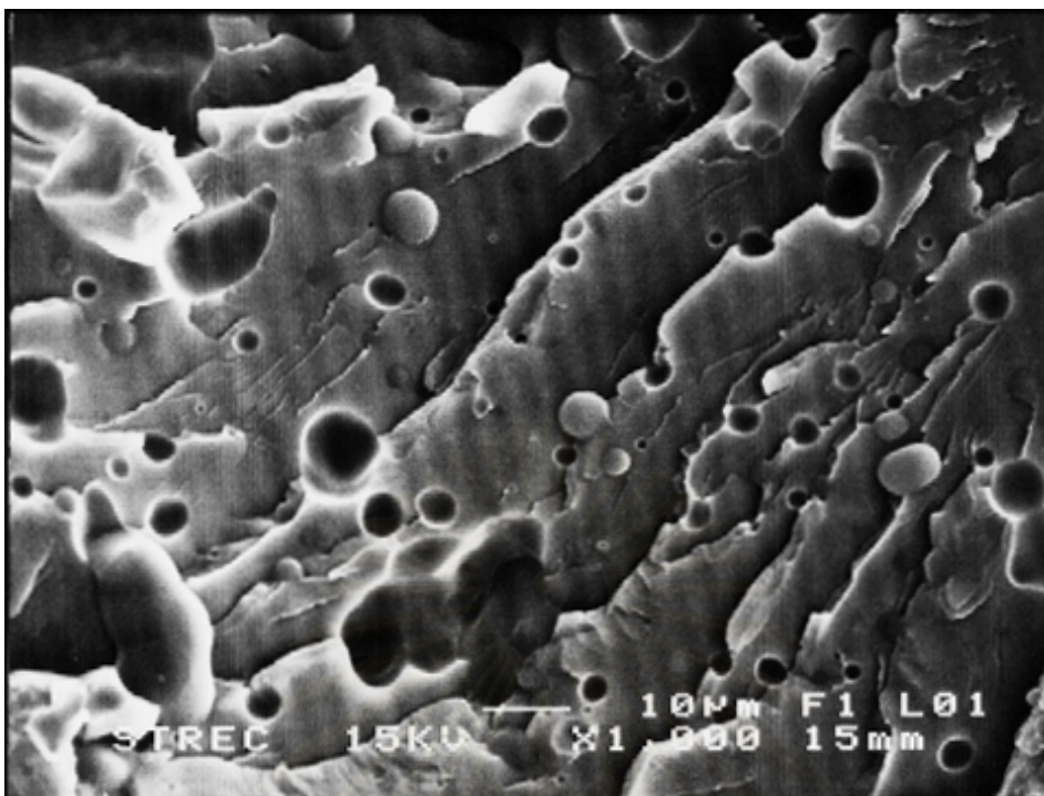
Figure 4.14 Scanning electron micrograph of PET/Buna3950 blend at 80/20, using 5 phr MAH grafted onto EPDM.
