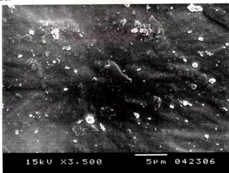
Figure A26 SEM micrograph of PU/PS elastomer at the equivalent weight ratio of MDI:POLYOL:TAPE = 2:1.4:0.6, 20 wt% of styrene, and 2 wt% of MEKP/Co.
