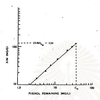
Figure 2.3 Adsorption isotherm of phenol on activated carbon
