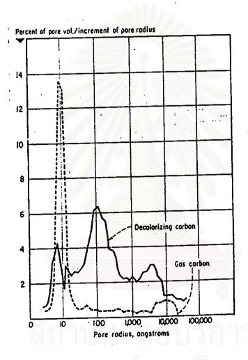
Figure 2.1 Comparison of pore volume distribution between liquid phase and gas phase activated carbon
