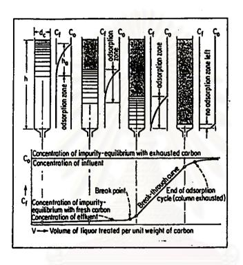
Figure 2.7 Adsorption zone depth and exhaustion-curve shape
