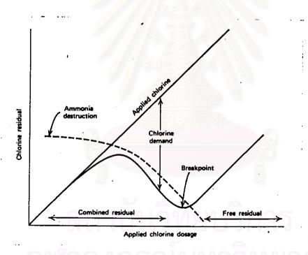
Figure 1.1. Typical breakpoint chlorination curve (2)
