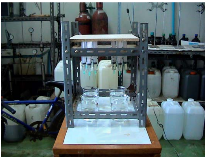
Figure 3.1 Chitosan beads preparation apparatus.
