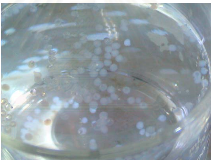
Figure 3.2 Chitosan form to gel beads in NaOH solution.
