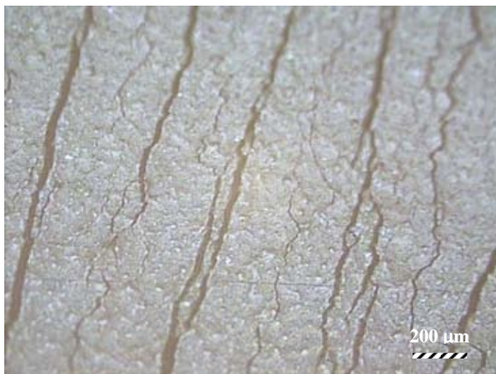
Figure 4.20 Cracks on the surface of stretched vulcanized NR film at the magnification of 10X.
