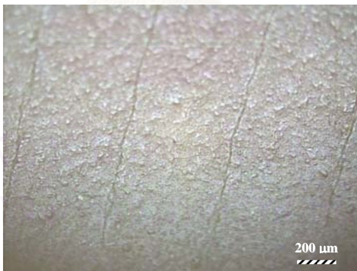
Figure 4.19 Cracks on the surface of vulcanized NR film at the magnification of 10X.
