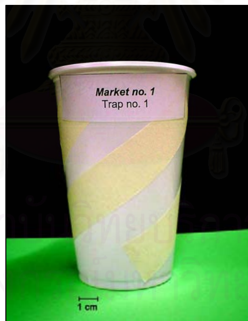
Figure 4.2 A modified jar trap was a plastic cup with the sticky crepe paper fixed around the trap for enabled cockroaches to enter, and a thin film of petroleum jelly was applied to the inner surface to prevent cockroaches escape.
