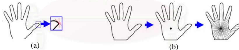
Fig. 4. The images show the general idea of (a) angle-based conversion technique and (b) centroid-based conversion technique.
