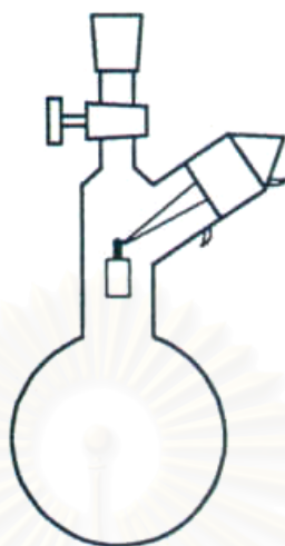
Figure 3.5. The special flask reactor for semibatch system
