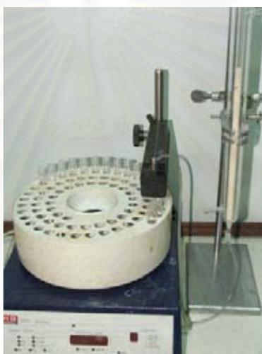
**Figure 3.3** Auto collecting sample from column
