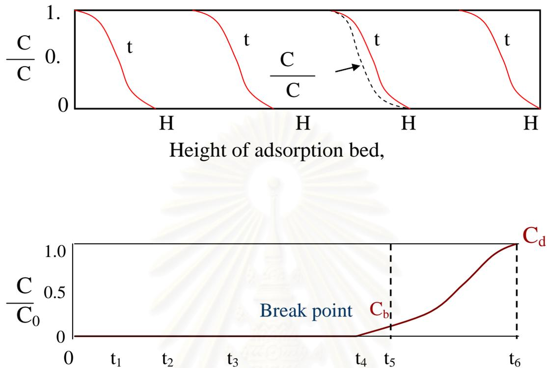
**Figure 2.3** Concentration profiles for adsorption in fixed bed (a) profiles at various positions and times in the bed, (b) breakthrough concentration profile in the fluid at the outlet of bed
