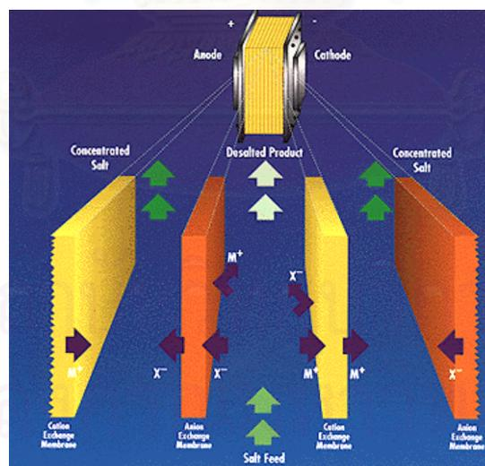
**Figure 2.4** Diagram of a typical ED cell
