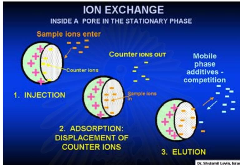
Figure 2.1 Mechanism of ion exchange
