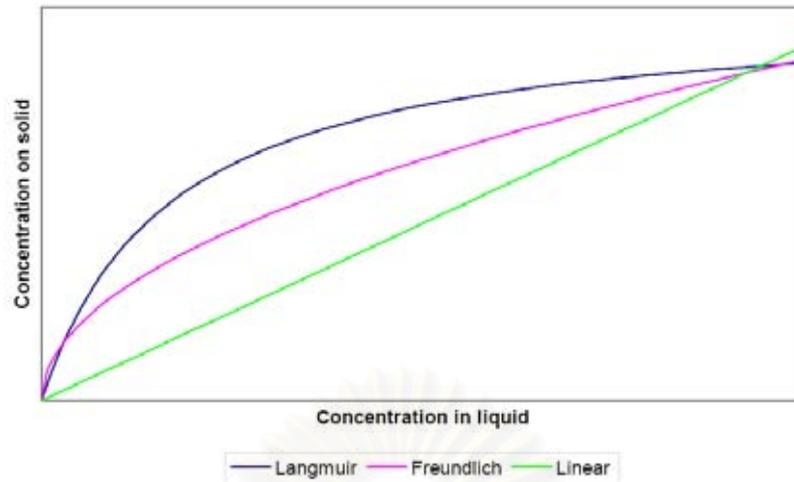
**Figure 2.2** Three common types of adsorption isotherms.
