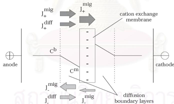
Figure 2.6 Concentration polarization
