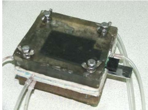
**Figure 3.4** The laboratory scale electro dialysis unit
