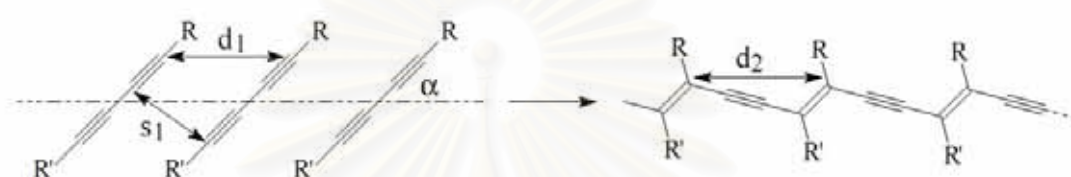
Figure 2.2 Schematic representation of topopolymerization of diacetylene monomers [8].
