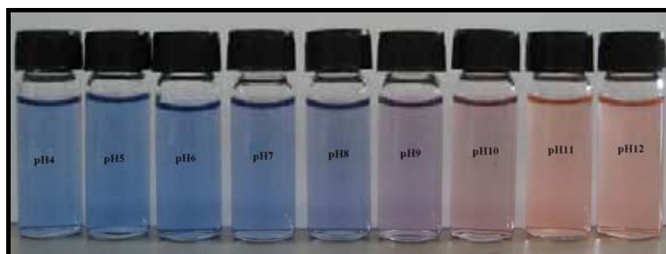
Figure 4.4 Photograph of pH induced color transition of PPCDA vesicles at room temperature.
