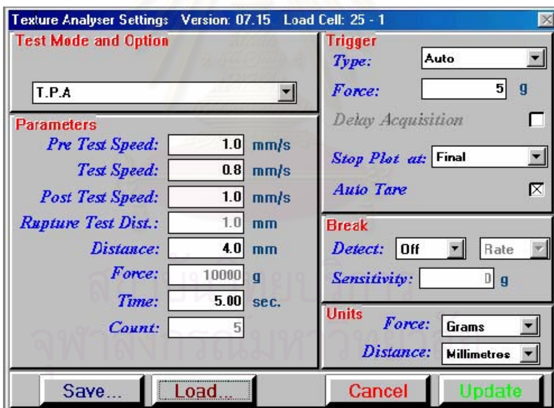
Figure 4.3 The conditions of texture analyzer for gel strength determination
