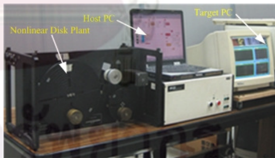
(ค) Matlab® xPC Real time Controller
