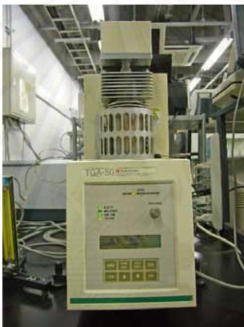
Figure 3.11 Thermogravimetric analyzer (TGA-50, Shimadzu).
