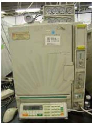
Figure 3.5 Gas chromatograph (Shimadzu, GC-14B) with TCD detector.
