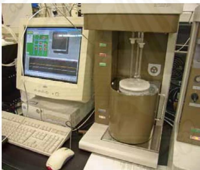
Figure 3.9 Analytical apparatus for N<sub>2</sub> adsorption (BEL Japan, Belsorp mini) which was used for determining BET specific surface area.
