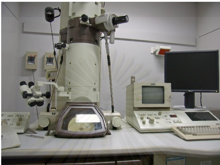
Figure 3.3 Transmission electron microscope (TEM; JEOL, JEM-1010).
