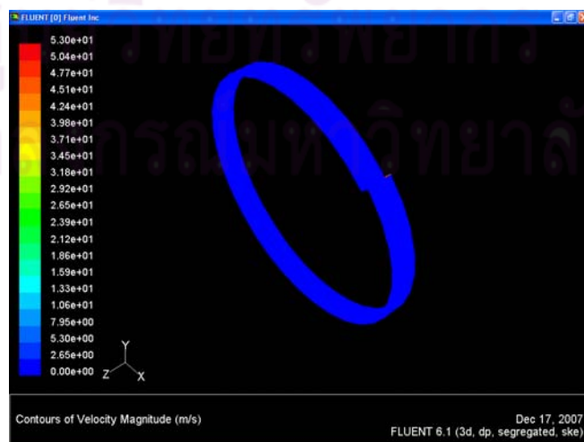
Figure 6.16 Velocity Contour of Water Test for Curvature Ratio 0.024
