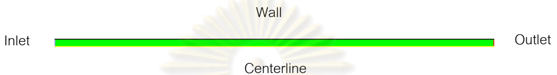
Figure 5.4 Boundary Conditions for Circular Pipe
