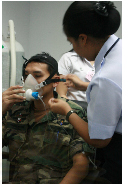
Figure 3.2 Fitting a one-way valved mask of Gas Analyzer
