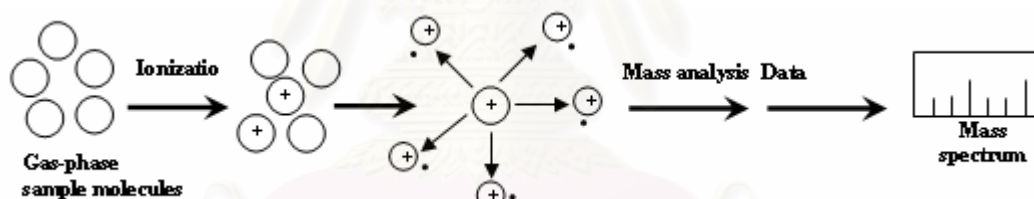
Figure 2.6 Basic concept of mass spectrometry analysis
