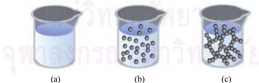
Figure 4.1: Progress of the reaction of RF solution: (a) solution (b) colloid and (c) gel.
