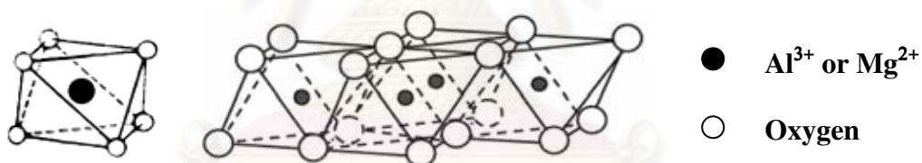
Figure 2.2 A single octahedral unit (a) and a sheet structure of octahedral unit arranged in a hexagonal network (b) [18].
