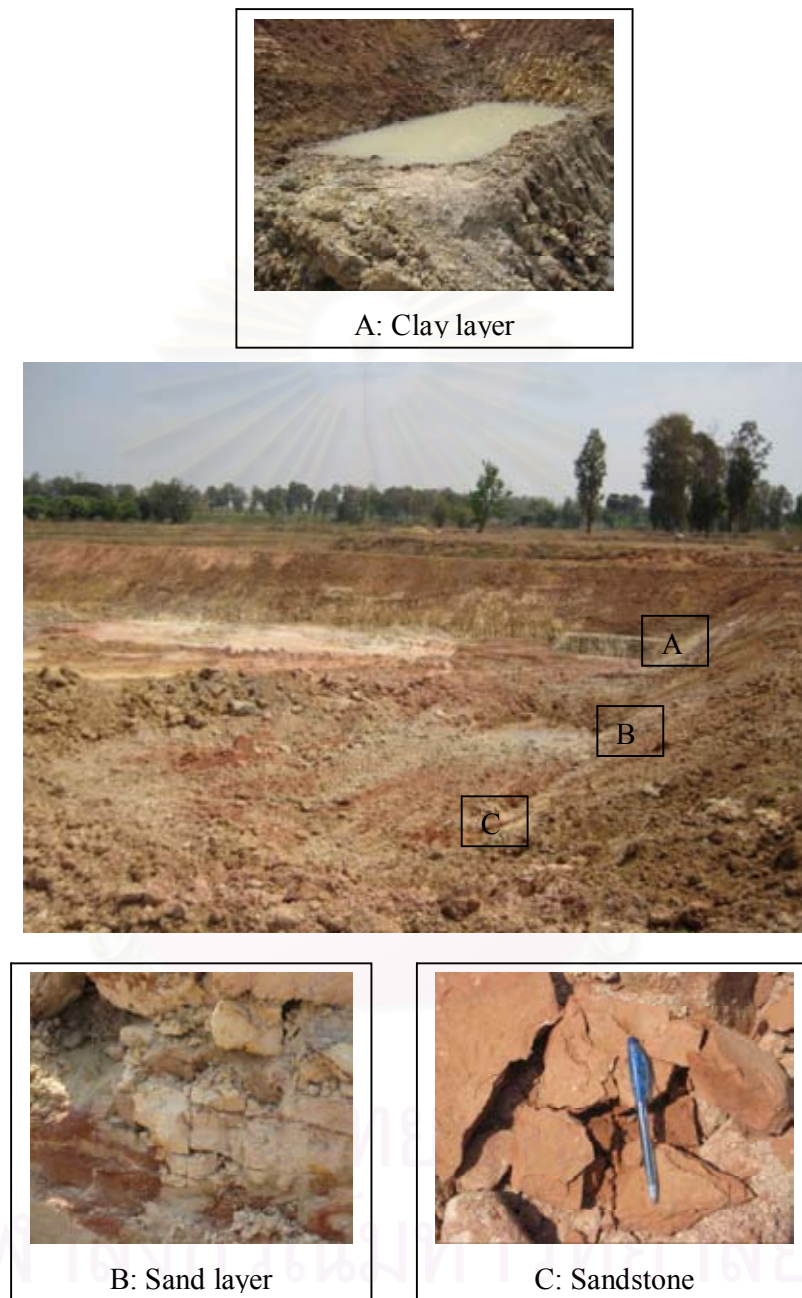
Figure 4.36 Soil profile and rock type of the areas closed to the preferred site.
