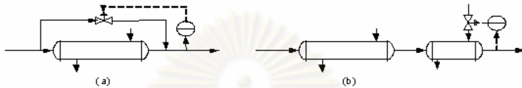
Figure 3.9 Control of P/P heat exchangers: (a) use of bypass; (b) use of auxiliary utility exchanger.
