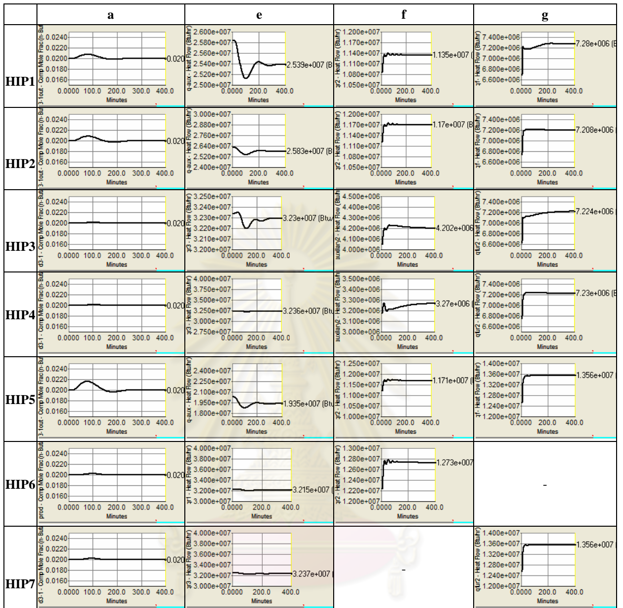
Figure 5.69 Dynamic responses of the Butane Isomerization plant CS 1 to increase in recycle flow from 870 to 940.1 lb-mol/h; comparison between CS1, CS2, CS3, CS4, CS5, CS6, CS7 and CS8, where (a) product composition, (e) reboiler duty of DIB column, (f) reboiler duty of Purge column, and (g) furnace duty.
