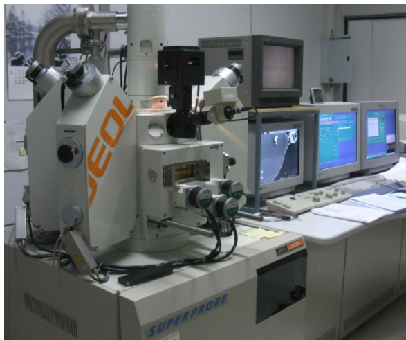
Figure 1-2 Electron Probe Micro Analyzer (EPMA), Model JXA-8100 based at Department of Geology, Faculty of Sciences, Chulalongkorn University.
