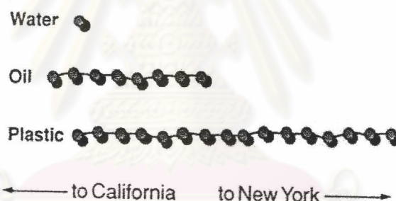
Figure 2.1 The length of the carbon chain in plastic compared to that in water and oil.
