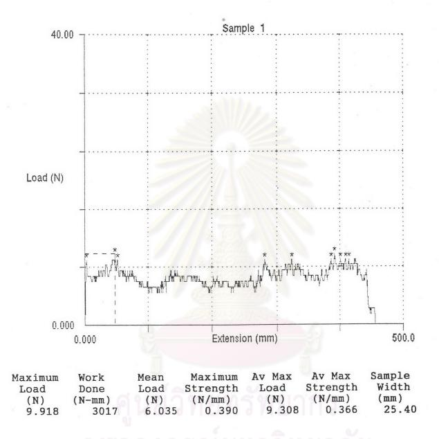
FIGURE 6.1 Peel tension graph of sample 1
