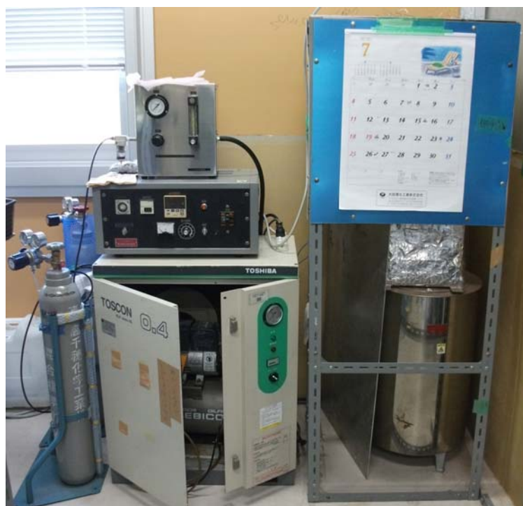
Figure 3-7. Sand bath with batch type reactors put inside.
