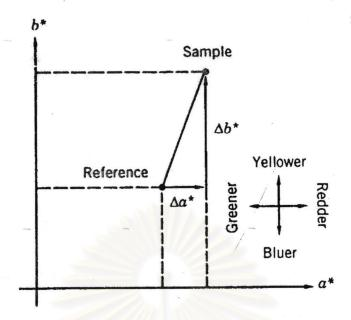
Figure 2-4 Resolution of the chromaticity difference into  $\Delta a^*$  and  $\Delta b^*$  in the CIELAB system
