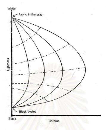
Figure 2-6 Constant loci of colour depth and dyer's brightness on a plot of lightness against chroma
