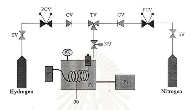
Figure 3.1 Schematic drawing of the reaction unit
