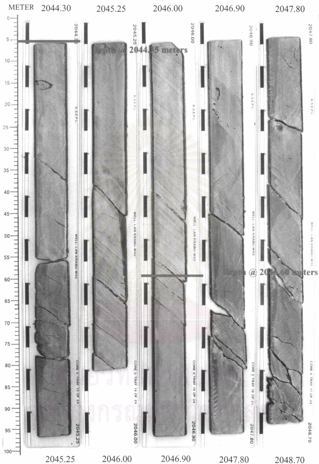
Figure 3.4 Lithofacies CS shows claystone interlaminated and interbedded with light grey sandstone and siltstone (sample LKU-W02 at depths between 2044.35 and 2046.60 meters).
