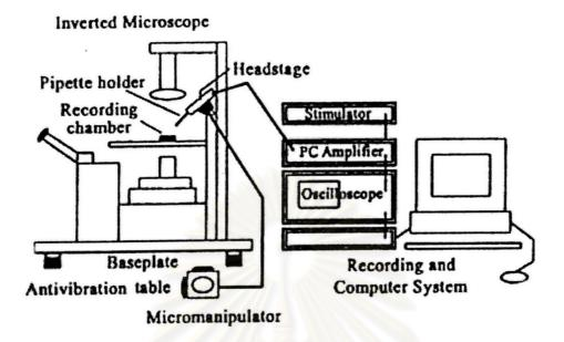
Figure 6 Diagram for the whole-cell application of the patch-clamp technique.
