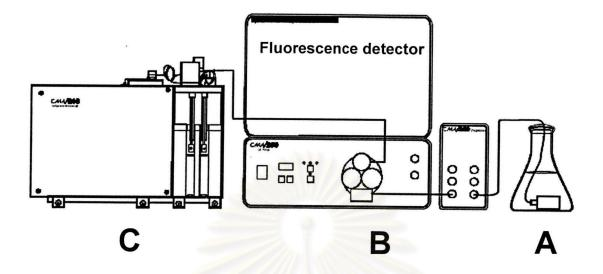
Figure 5 Diagram for HPLC system with mobile phase (A), HPLC Pump (B), Sample injector (C) and Fluorescence detector.
