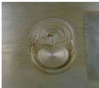
Figure 3-7 The OLDE_01 dented electrode for toner supplying
