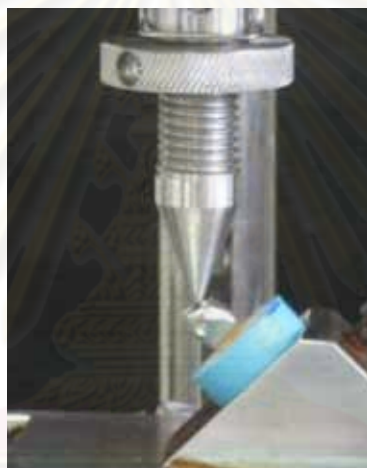
Figure 11. Specimen mounted at 135 degrees in Instron Testing Machine.
