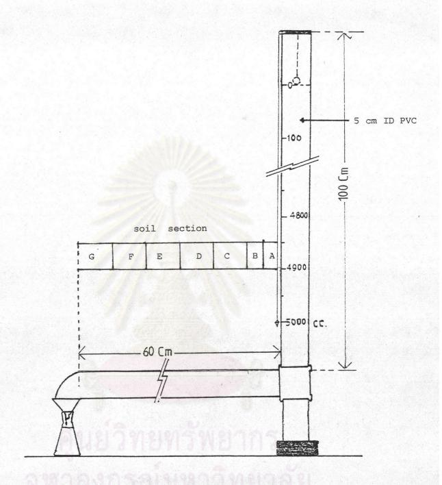
Figure 3.2 Typical soil column that used in this experiment
