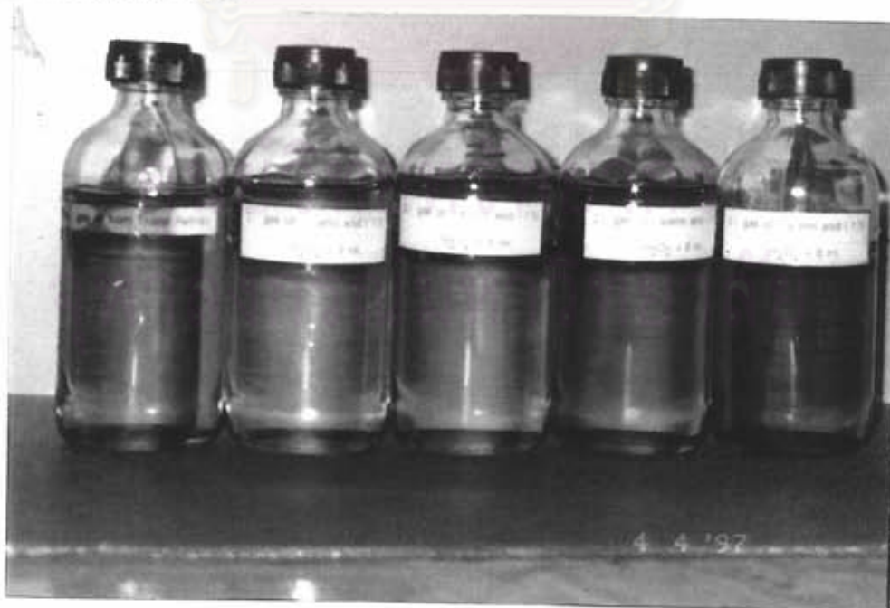
Fig. 4.2 Effect of hydrogen peroxide as oxidant to colour of high speed diesel.
