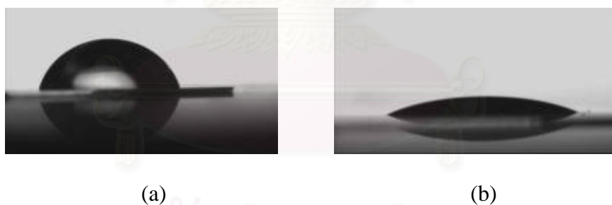
Fig. 2.2 Appearance of contact angle of (a) before irradiation of UV light, (b) after irradiation of UV light
