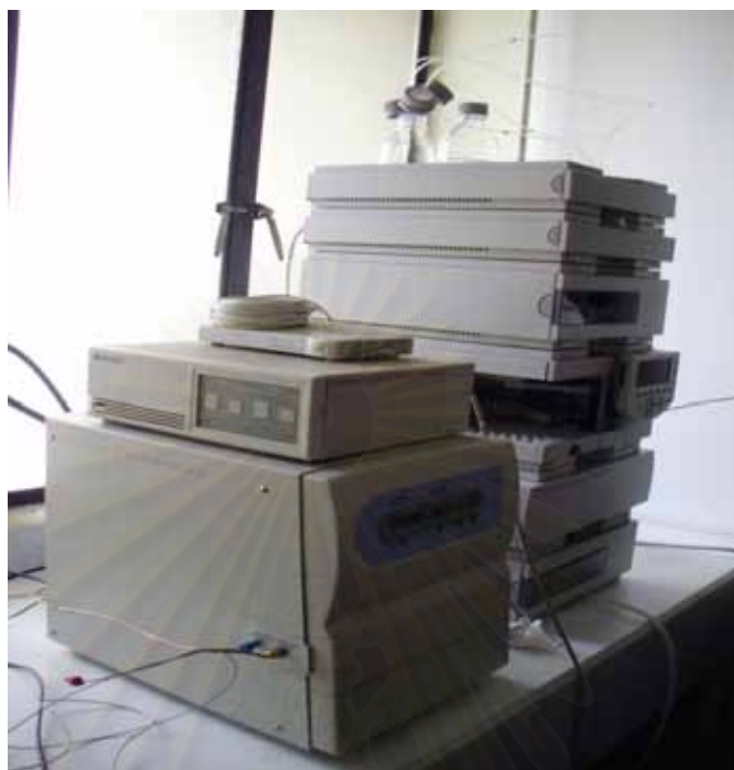
Figure A-3 The High Performance Liquid Chromatography (HPLC 1100, Agilent) with ELSD and UV detector
