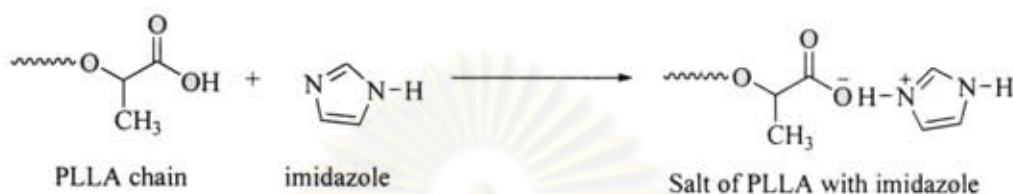
Scheme 4.7 Formation of PLLA salt with imidazole
