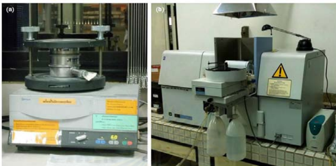
Figure 11 Model for determination of acid-soluble arsenic content. (a) Material was pulverized and passed through 75-micron sieve (b) Atomic absorption microscopy model AAAnalyst 800.
