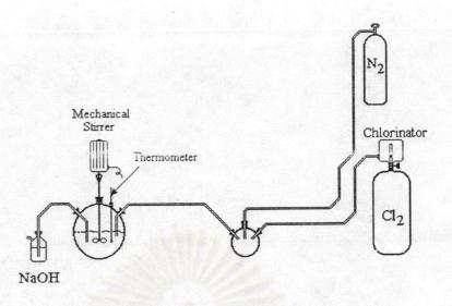
Figure 3.1 Apparatus for chlorination
