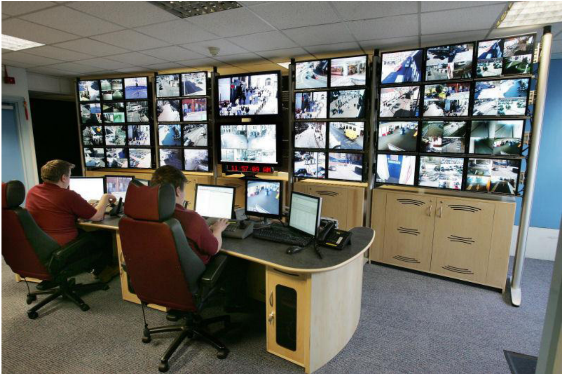
Figure 1.1: Conventional video surveillance system that involves with an operation on human abilities.
