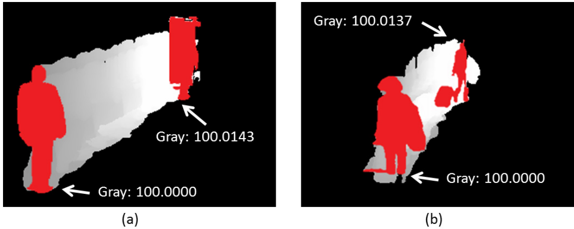
Figure A.3: Back view tunnels in time-space show the gray value was assigned differently in the decimal part. As you can see, we set a flag value of integer part to be 100, and the decimal part is depends on the slice number inside a tunnel.
