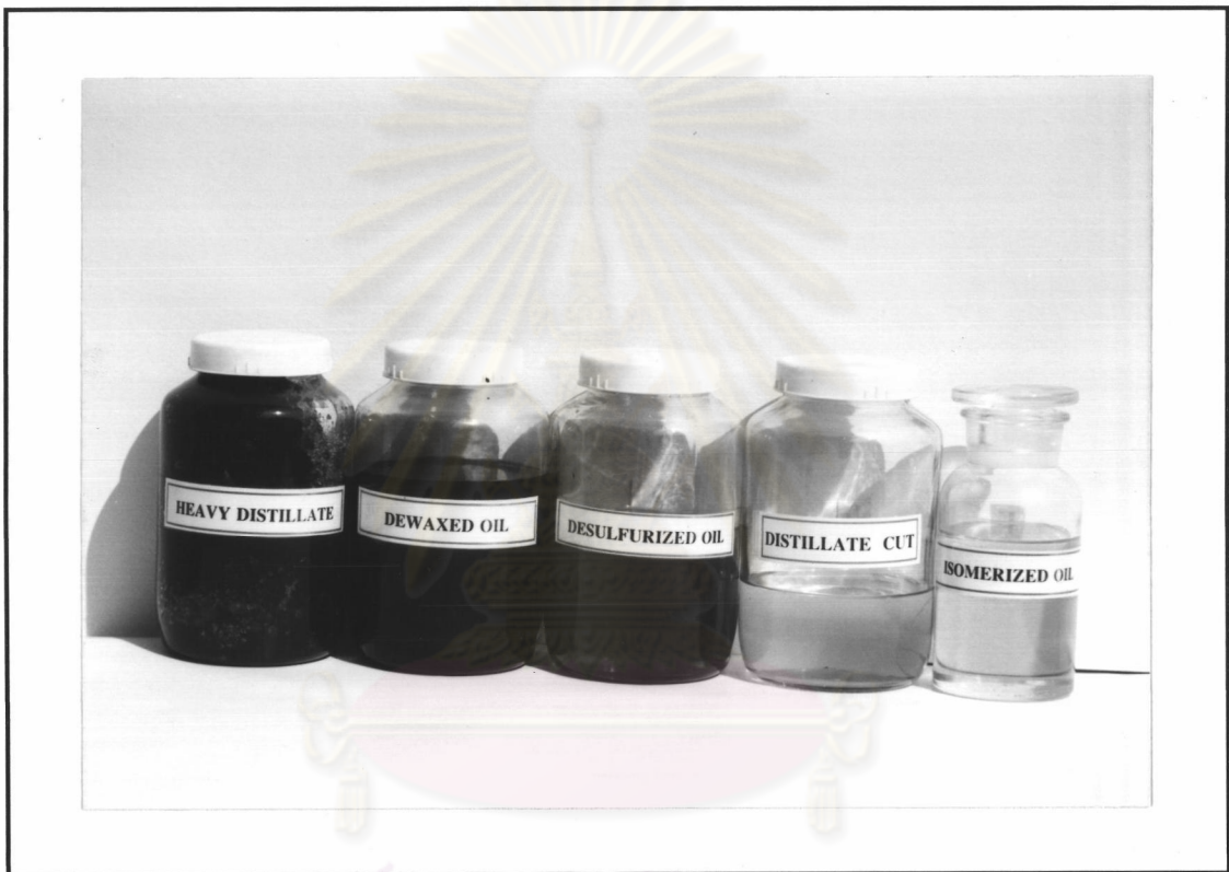
Figure 4.34 Heavy distillate, dewaxed oil, desulfurized oil distillate cut, and isomerized oil at the optimum conditions for each processing step
