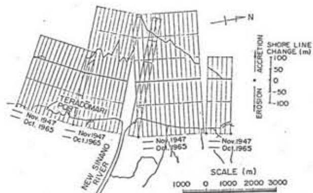
Fig. 8 Shoreline changes at the coast around the mouth of the New-Shinano River.
