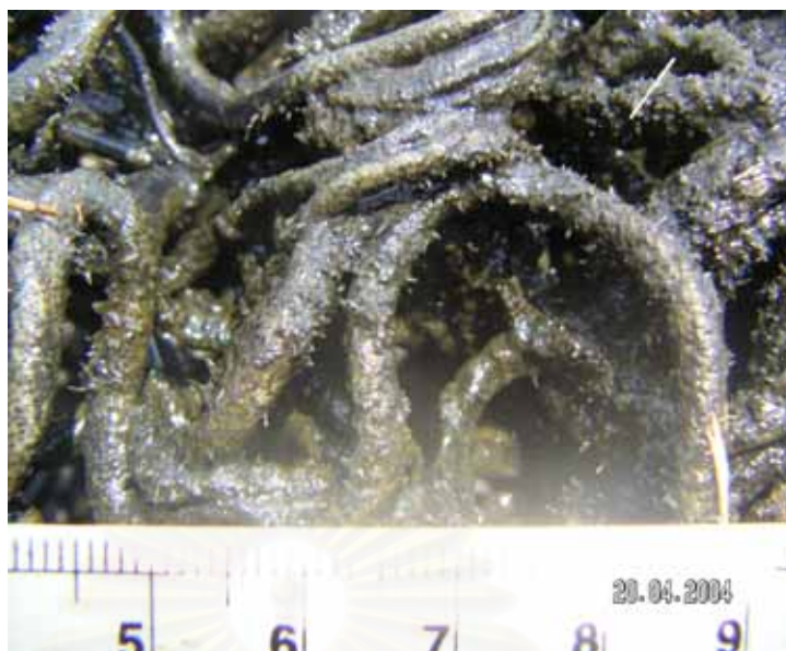
Figure 4-3: One month-old biofilter coated with sludge and biofilm
