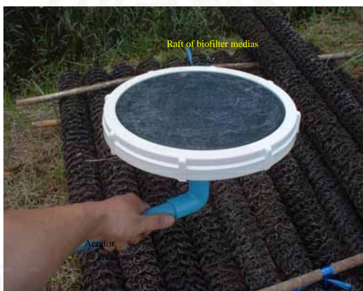
Figure 3-5: Biofilter (cylinder-shape porous plastic tubes) and aerator disc before being installed in the pond.
