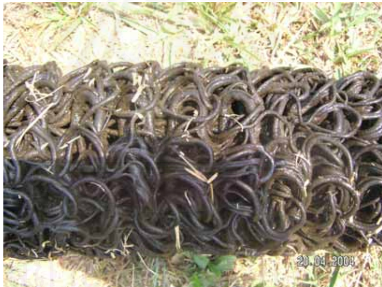
Figure 3-1: The Hyper Drain™, a polypropylene biofilter media used in this study
