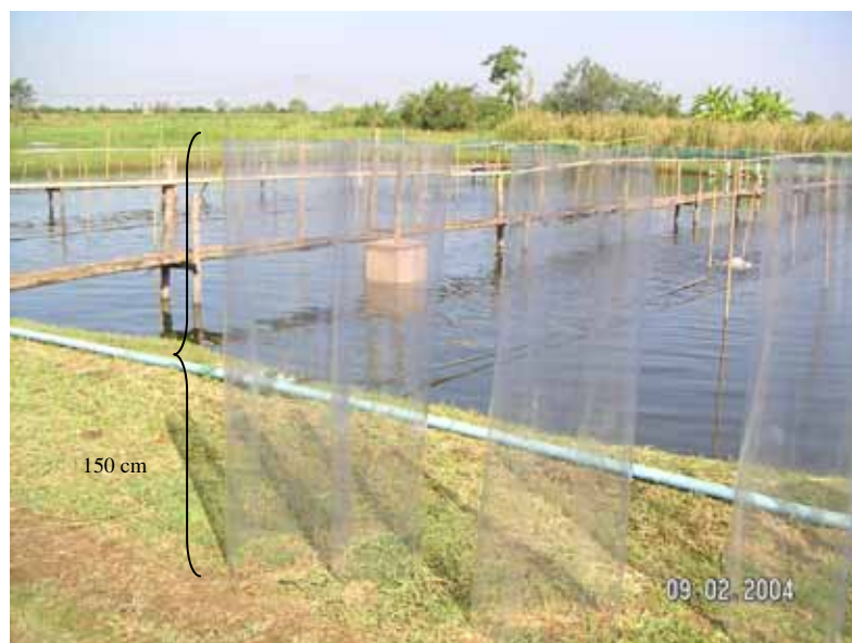
Figure 3-3: The custom-made clear PVC tubes used in the field experiment.
