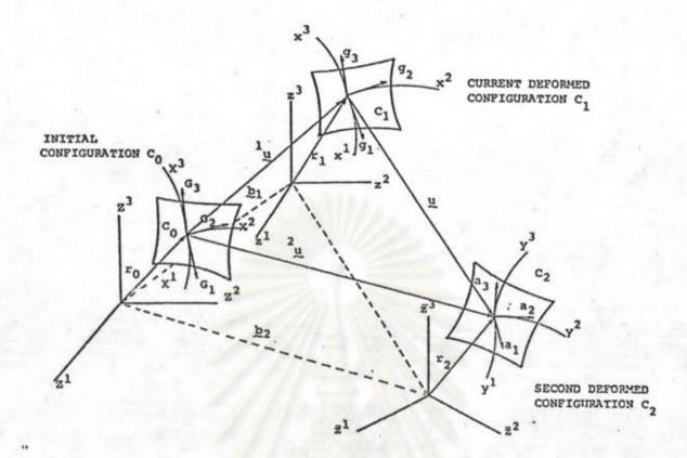
FIGURE 2.1 Deformation Path of a Body.
