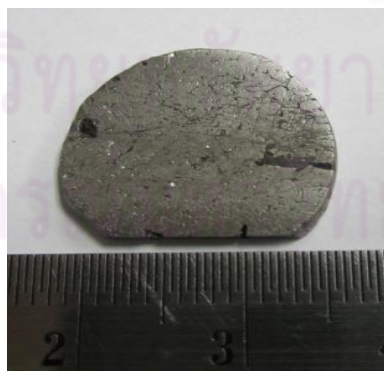
Figure 4.4: Disk shape of FeSi_x after cutting by precision diamond saw prepared for thermal diffusivity measurement.
