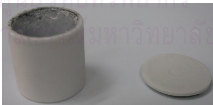
Figure 3.5: Alumina crucible and cover coated with boron nitride releasing agent.
