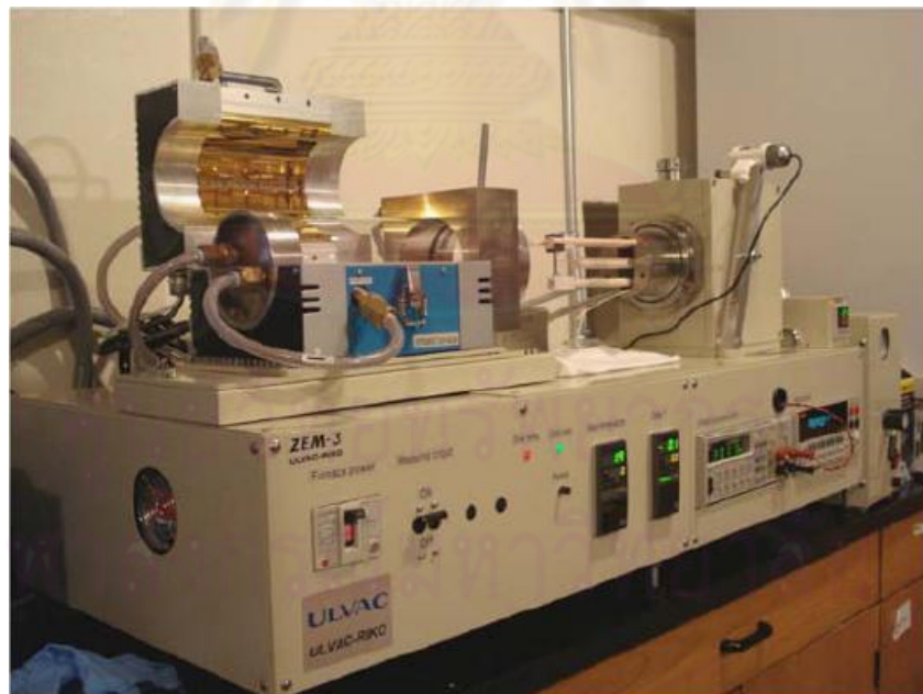
Figure 3.20: The commercial equipment (ZEM-3, Ulvac, Inc.) is used to measure the electric resistance and Seebeck coefficient from room temperature to 700 °C. [48]
