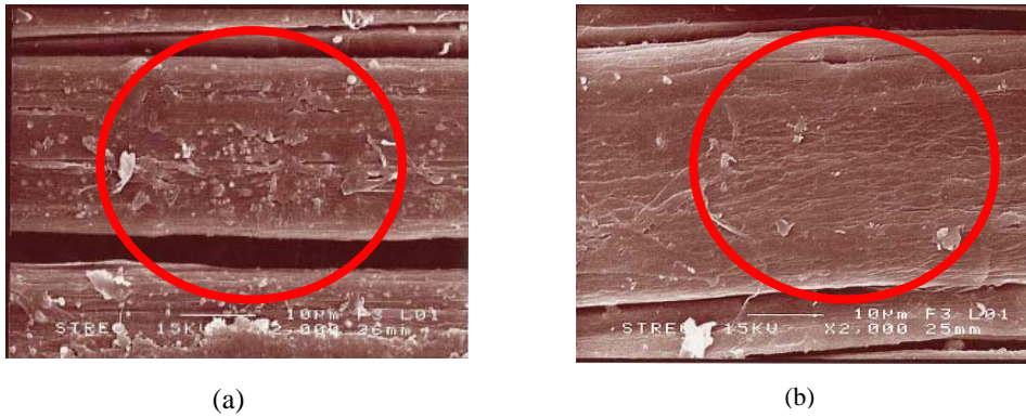
Figure 4.1 SEM micrographs of hemp fabric (a) untreated, (b) treated with 5% NaOH
