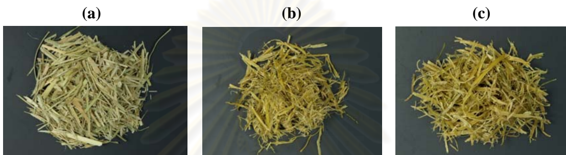
Figure 3.1 Vetiver grass fiber (a) Untreated (b) Mercerization treated and (c) Silane coupling agent treated.
