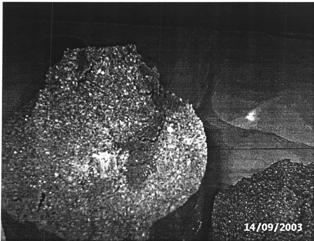
QVF 05 10% of Bentonite Content – Overburden Stress = 200 kPa
