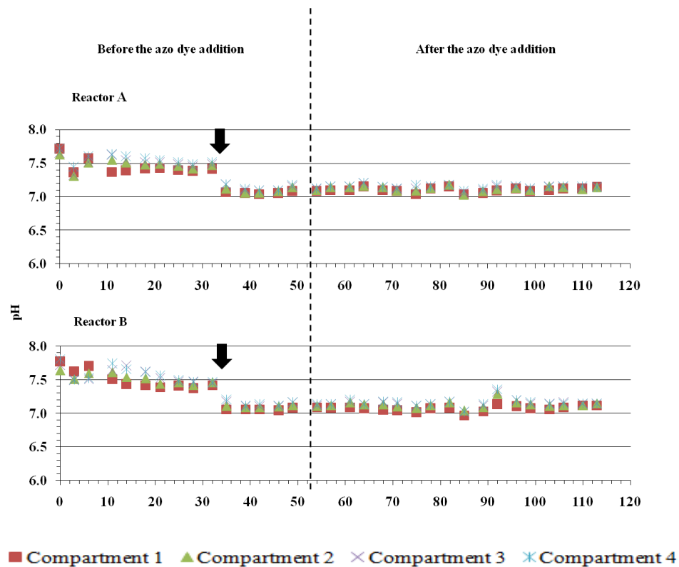
Figure 4.4 pH values in each compartment of Reactor A and Reactor B: ( ↓ ) after 34 days of the experiment, the pH in synthetic wastewater was adjusted to pH ~7, ( - - - ) line for separation between before and after the azo dye addition on day 53 th
