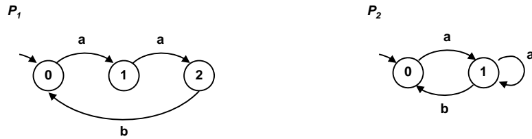
Figure 2.1: Example of LTS P_1 = \langle S^1, \Sigma^1, \Delta^1, s_0^1 \rangle (left) and LTS P_2 = \langle S^2, \Sigma^2, \Delta^2, s_0^2 \rangle (right) with \Sigma^1 = \Sigma^2 = \{a, b\} .
