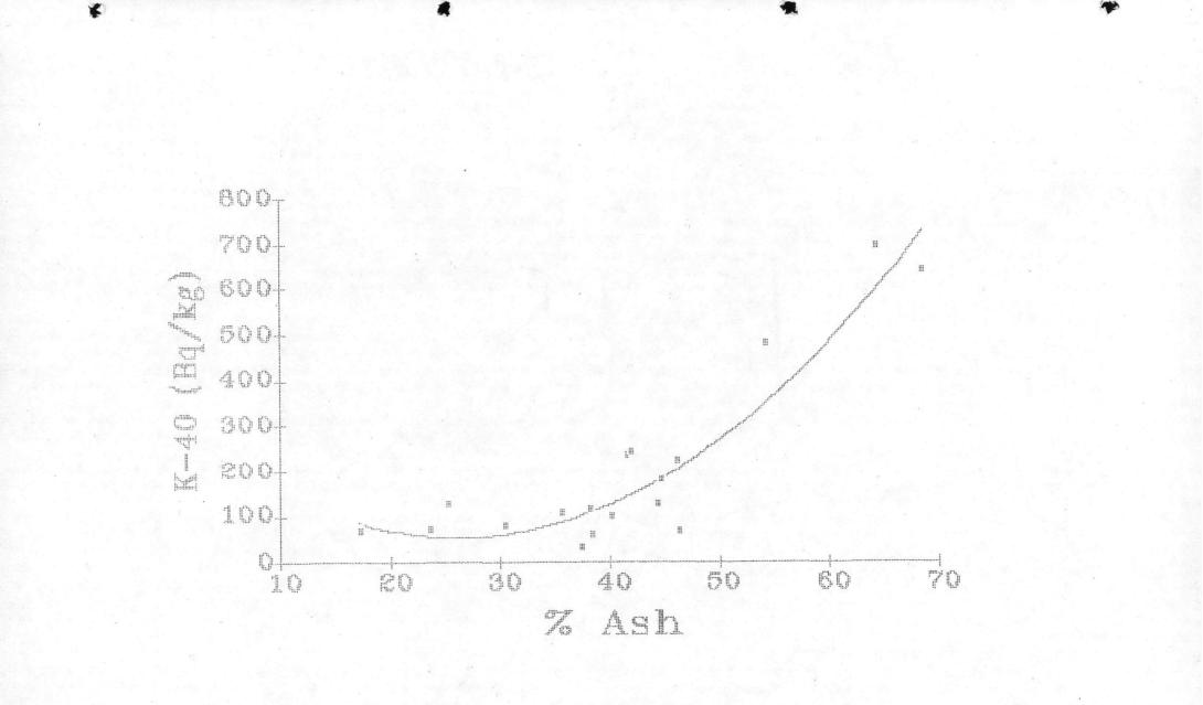
Figure 4.3 K-40 Activity in Lignite VS % ASh
